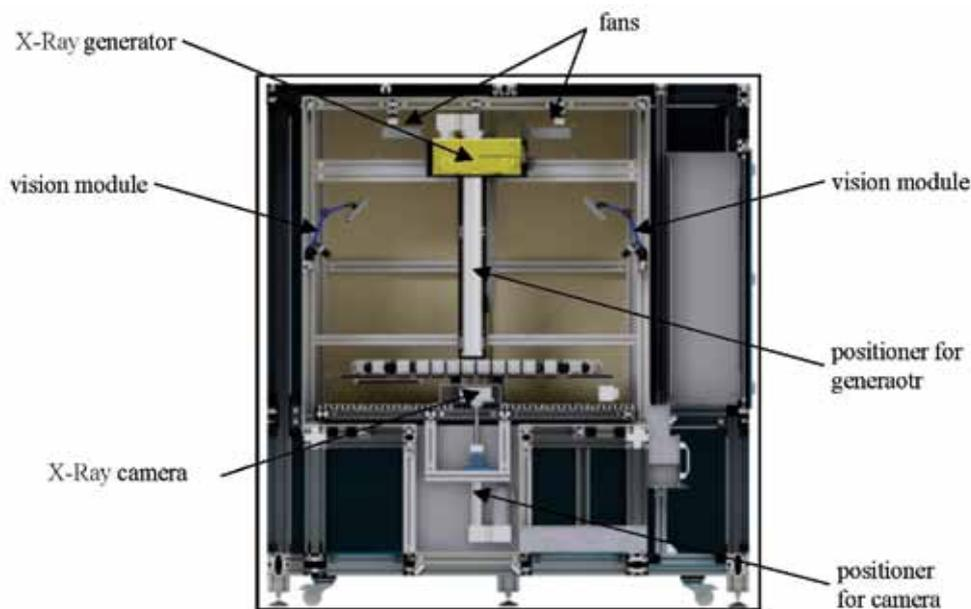
Fig. 2. General view of the inner chamber
