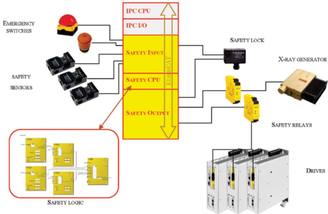
Fig. 8. Structure of safety systems
