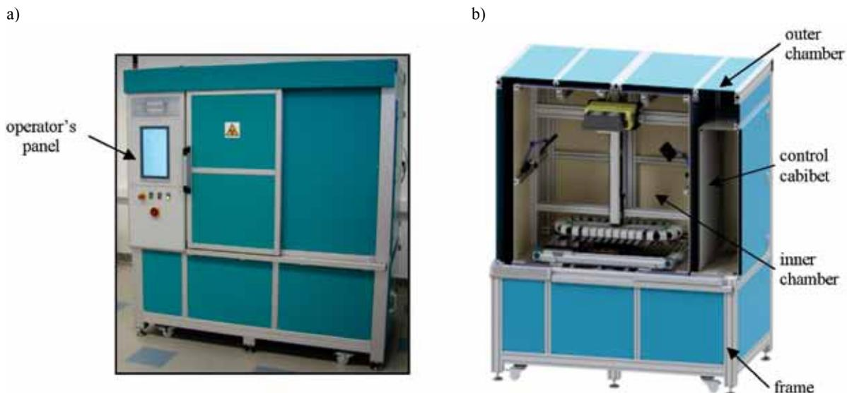
Fig. 1. The research system for X-Ray imaging methods: a) general view of the system, b) cross-section of the 3D model showing the internal measurement chamber
