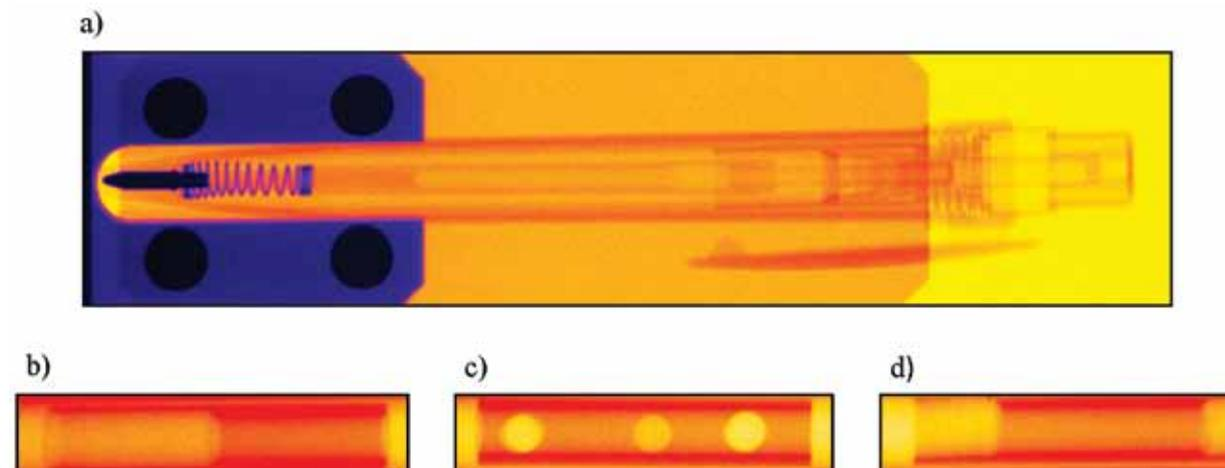
Fig. 11. Samples of registered images: a) ball pen, b) sleeves broached from the left side, c) sleeve with through-bores on both sides, d) sleeves broached from both sides
