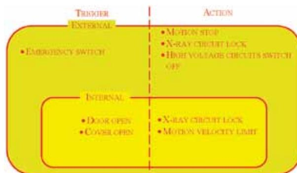
Fig. 7. Schematic diagram of the operation of safety systems
