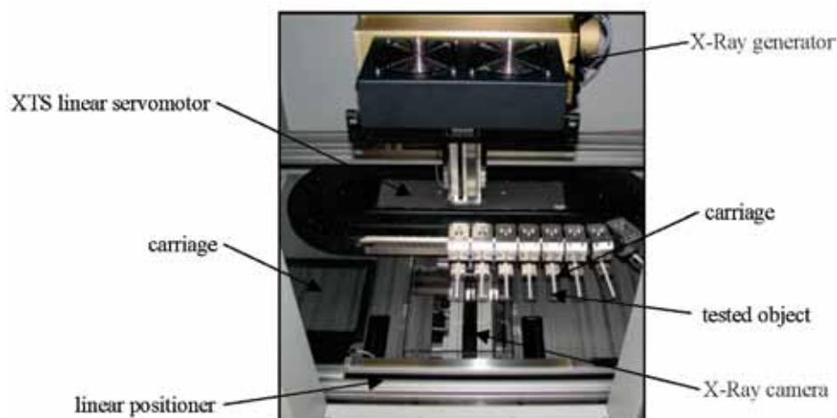
Fig. 3. The view of the filter segment inspection system
