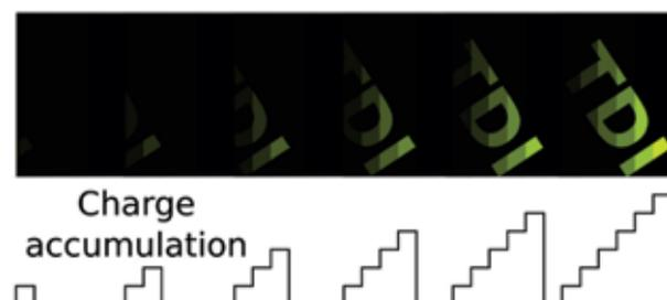
Fig. 10. Principle of operation of TDI mode [15]
