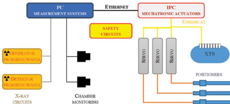
Fig. 5. Block diagram of device control systems
