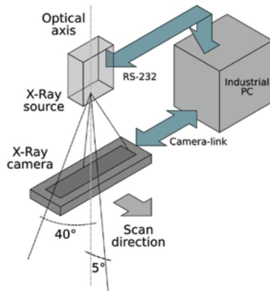
Fig. 9. X-Ray beam geometry and image acquisition system
