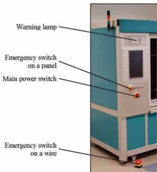
Fig. 6. Arrangement of security system controls
