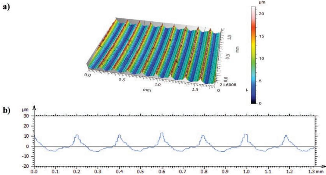
Fig. 5. Surface texture of the edge of the workpiece after dry turning with a cemented carbide cutting tool: a) isometric view, b) primary profile
