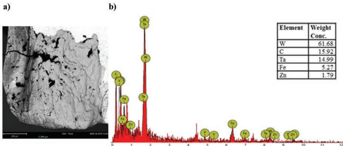
**Fig. 9. ISEM analysis of the tool wear made of cemented carbides after turning with cutting fluid containing zinc aspartate: a) image of the wear track and b) X-ray energy spectrum**
