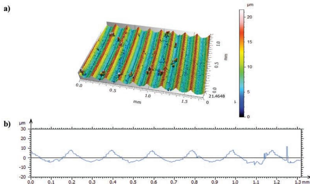
Fig. 8. Surface texture of the edge of the workpiece after turning with cutting fluid containing zinc aspartate with a cemented carbide with a-C:H coating cutting tool: a) isometric view, b) primary profile
