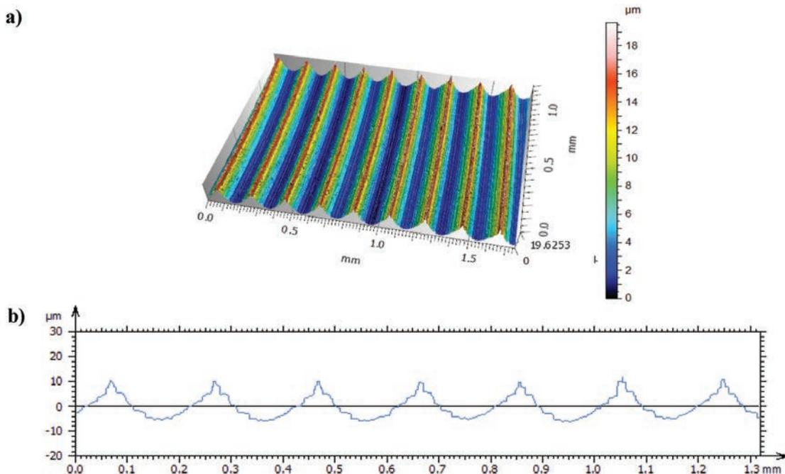
Fig. 6. Surface texture of the edge of the workpiece after dry turning with cemented carbide cutting tool with a-C:H coating: a) isometric view, b) primary profile
