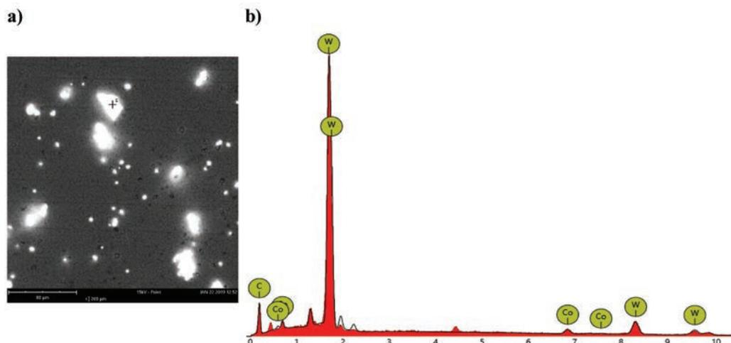
Fig. 3. SEM image: a) surface morphology, b) characteristic spectrum (EDS) in a micro-area for a diamond-coated cemented carbide insert
