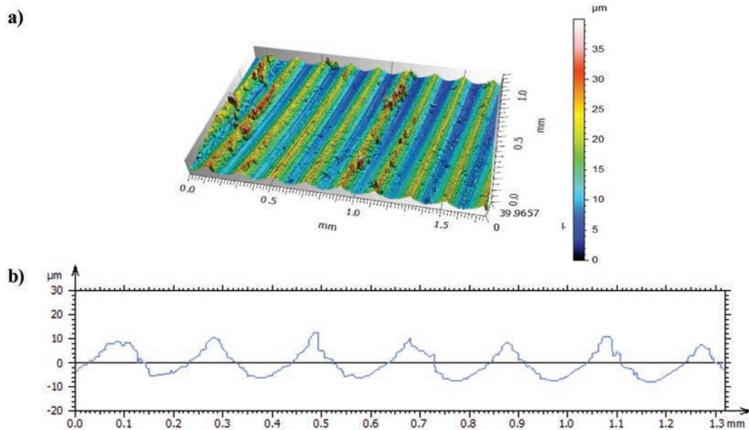
Fig. 7. Surface texture of the edge of the workpiece after turning with cutting fluid containing zinc aspartate with a cemented carbide cutting tool: a) isometric view, b) primary profile
