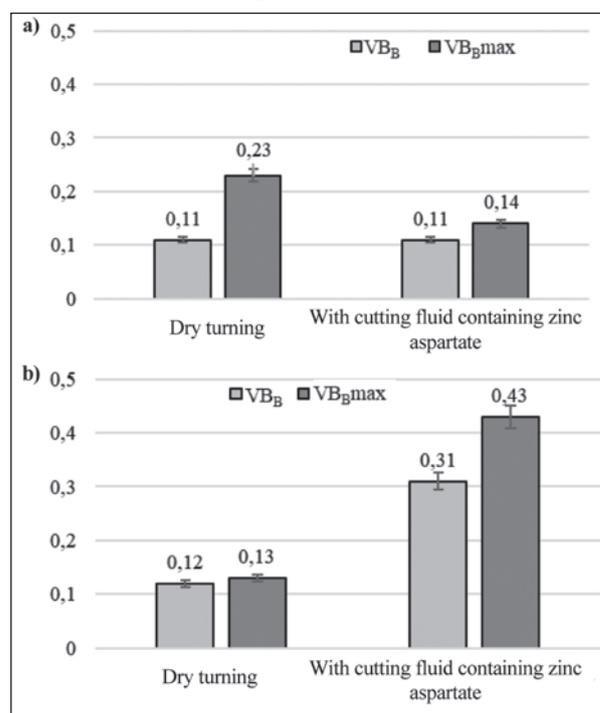
Fig. 4. Wear of the cutting tools made of cemented carbides after turning: a) without coating, b) with a-C:H coating
