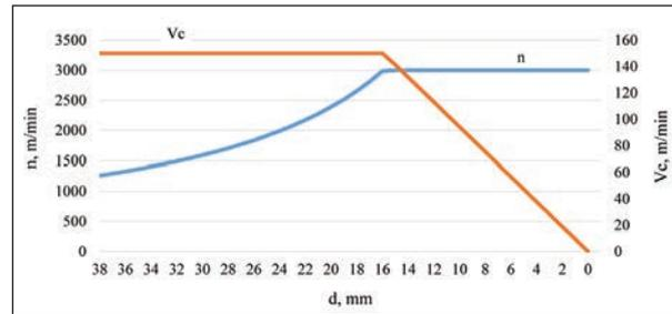
Fig. 1. Dependence of rotational speed and cutting speed on the turning diameter for cemented carbide tools without and with a-C: H coating
