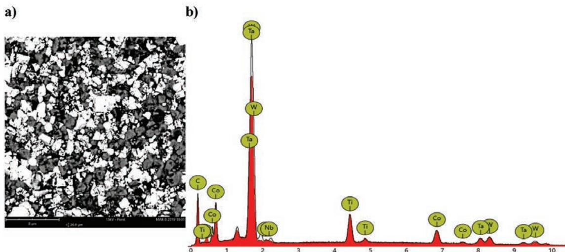
Fig. 2. SEM image: a) surface morphology, b) characteristic spectrum (EDS) in a micro-area for a cemented carbide insert
