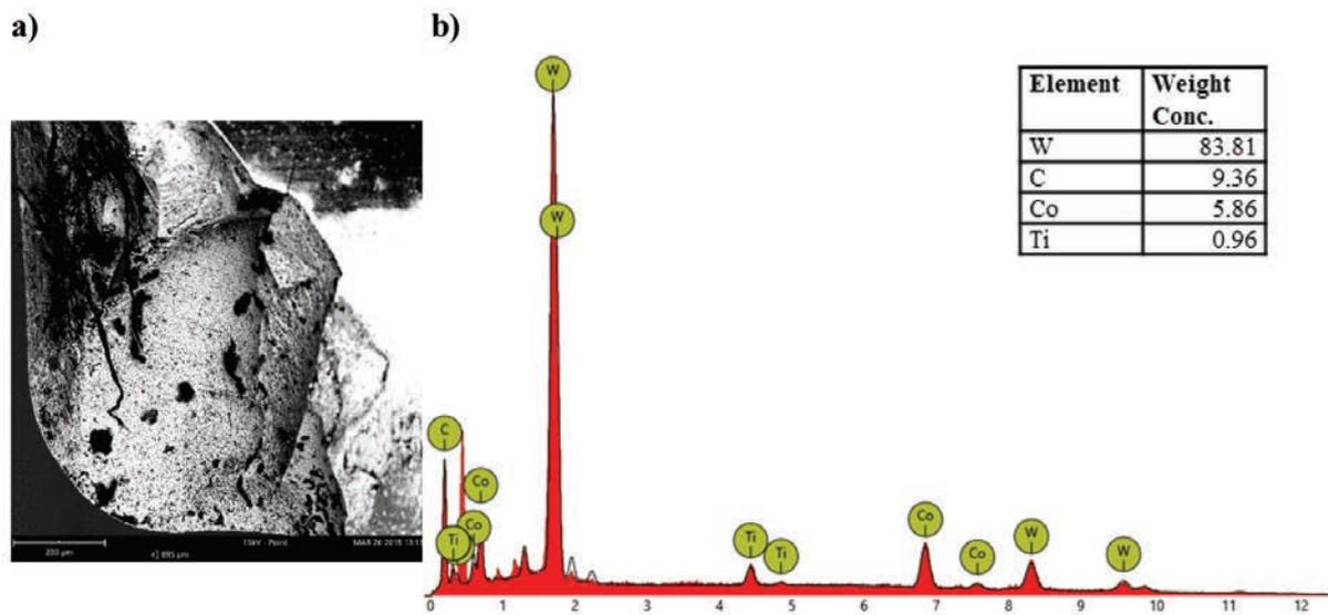
Fig. 10. SEM analysis of the tool wear made of cemented carbides with a-C:H coating after turning with cutting fluid containing zinc aspartate: a) image of the wear track and b) X-ray energy spectrum
