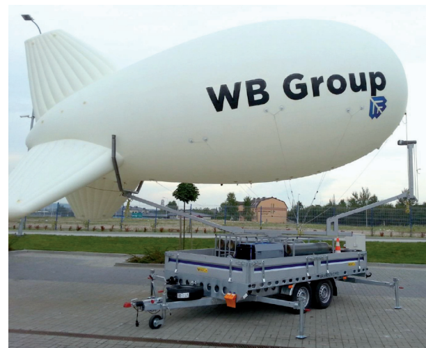
Fig. 2. Airship system skyRANGER docked in a mobile mooring station [22]
