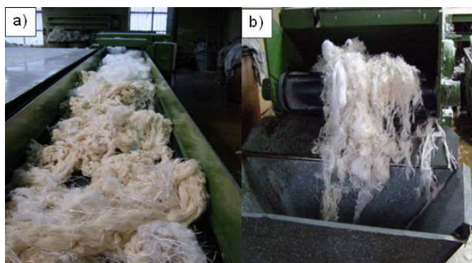
Fig. 3. Rotary cutter: a) input, b) output
