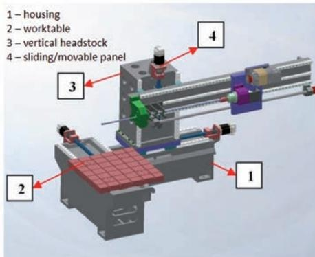
**Fig. 1. Virtual model of the designed machine WCZ 140**
