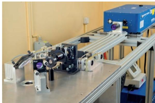
**Fig. 8. Prototype workstation for laser machining<sup>1</sup>**
