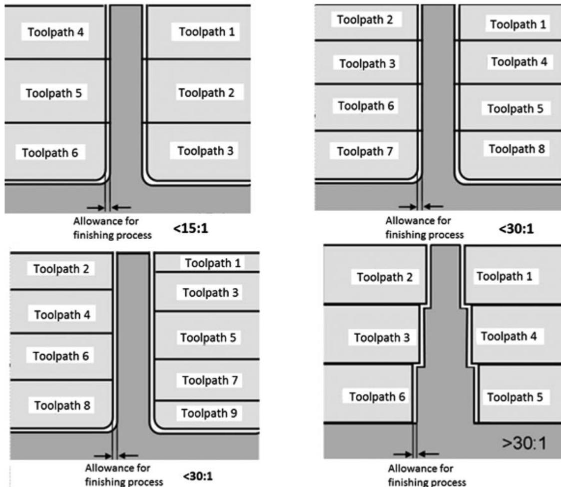
Fig. 7. Machining strategies of thin-walled elements depending on the height to thickness ratio of the milled wall
