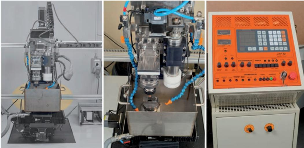
**Fig. 10.** Figures shows prototype workstation for electro-discharge micromachining with the mounting system of the workpiece, a bath for dielectric liquid, a power generator and a generator for programming the machining conditions<sup>2</sup>
