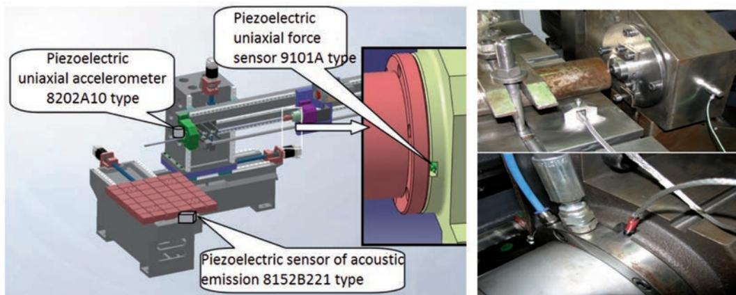
Fig. 4. The locations of sensors on the WCZ 140 drill during research
