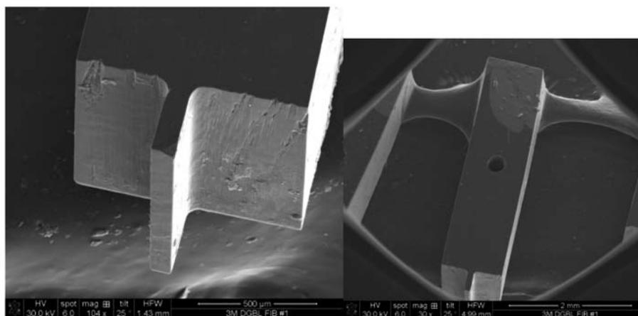
**Fig. 9. Examples of diamond microelements made on the workstation for laser machining [13]**
