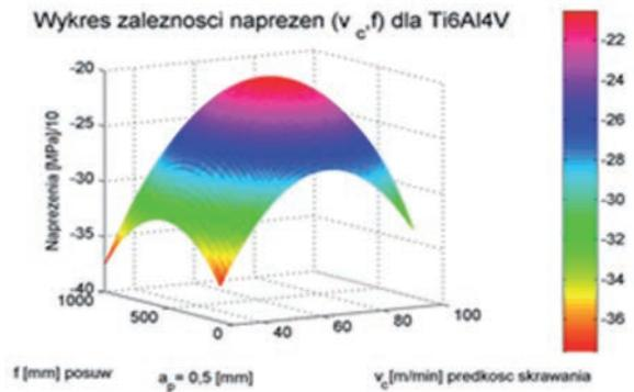
Fig. 16. The relationship between values of residual stresses measured in the perpendicular direction to the machined surface and cutting parameters (variable values of  $v_c$ ,  $f$ ) at constant depth of cut  $a_p = 0.5 [\text{mm}]$  for samples made out of Ti6Al4V
