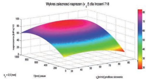
Fig. 17. The relationship between values of residual stresses measured in the perpendicular direction to the machined surface and cutting parameters (variable values of  $v_c$ ,  $f$ ) at constant depth of cut  $a_p = 0.5 [\text{mm}]$  for samples made out of Inconel 718
