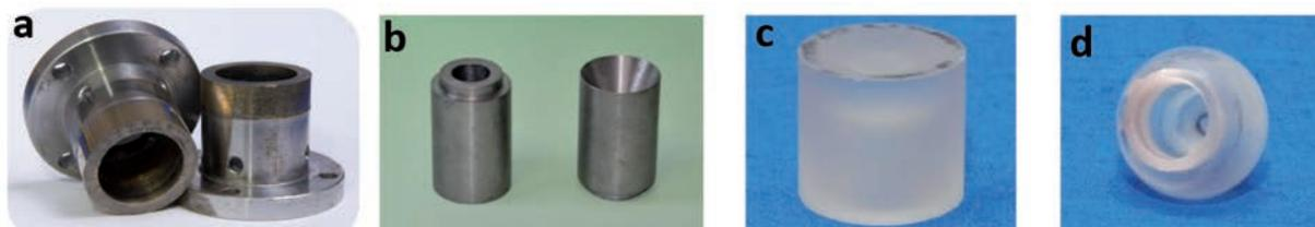
Fig. 14. Special tools: a) for preliminary machining of spherical elements, b) lapping iron for finishing machining, c) semi-finished product made out of single crystal sapphire, d) finished product
