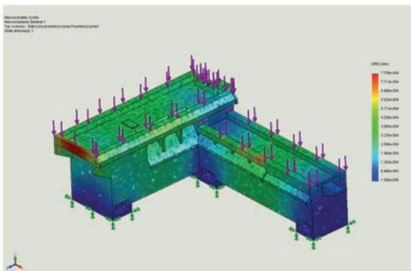
**Fig. 2. The analysis of the movement distribution of the housing under the load of cutting forces and weight**
