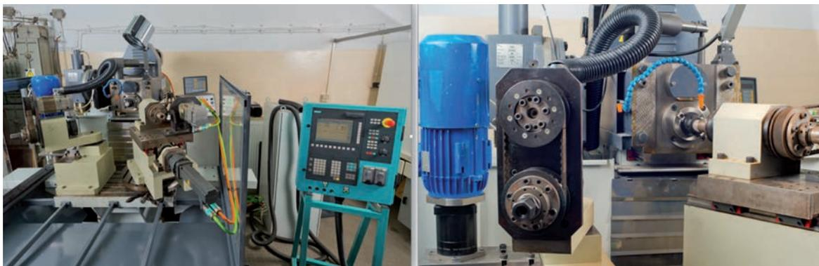
Fig. 13. The prototype workstation for machining of spherical ceramic elements, a) the workstation with the control system, b) a module for preliminary machining
