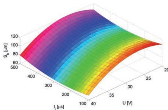
**Fig. 12.** The relationship between the thickness of the side gap, pulse time, of the duration impulse and interelectrode voltage U
