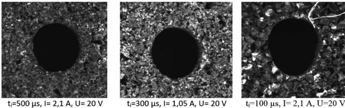
**Fig. 11.** Examples of the holes drilled in B,C carbide for different input machining parameters: pulse time, I – current intensity, U – interelectrode voltage
