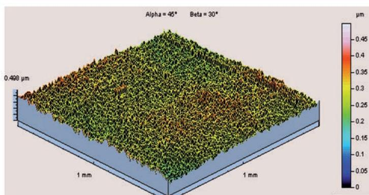
Fig. 15. The roughness of a spherical element after the finishing machining process performed by lapping iron and with a diamond micropowder abrasive paste
