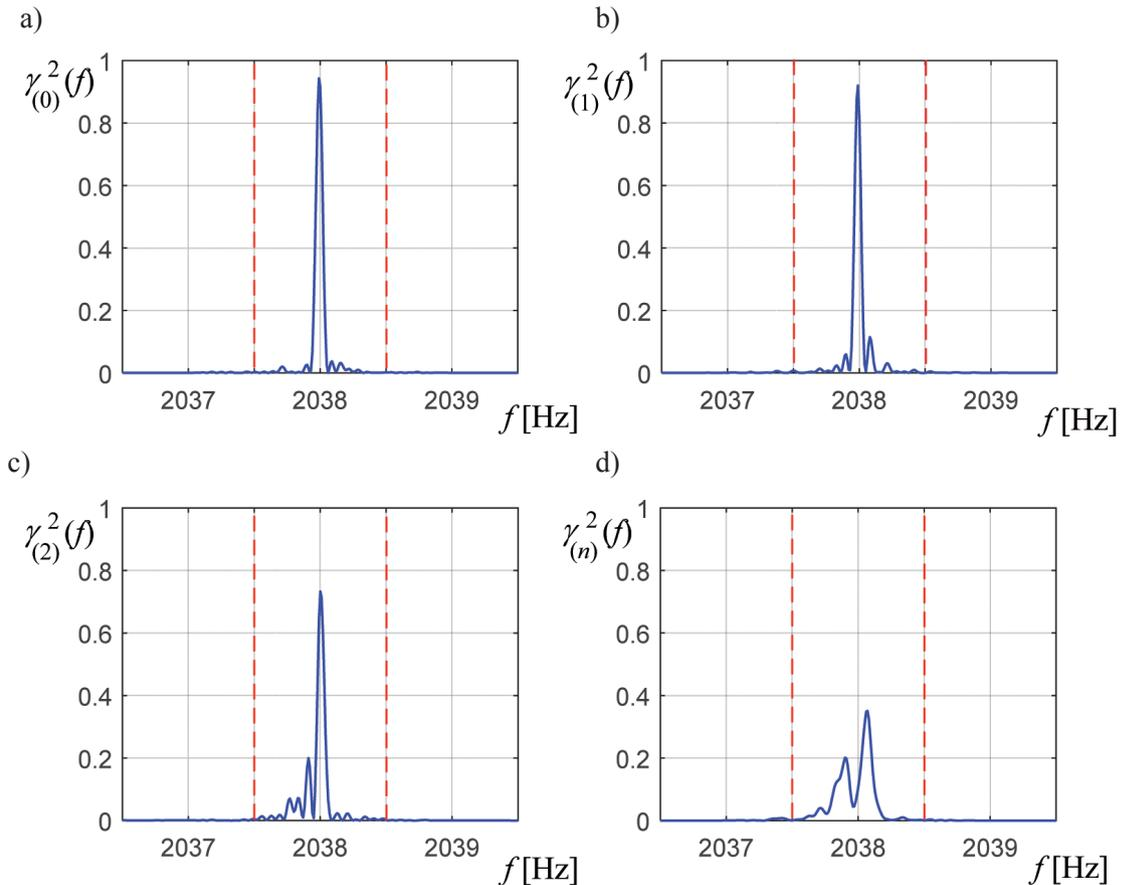
Fig. 7. Coherence function in the selected band: a) maintenance state without defects, b) maintenance state with a slightly defected tooth, c) maintenance state with a strongly defected, d) maintenance state with a new wheel (not run-in)
