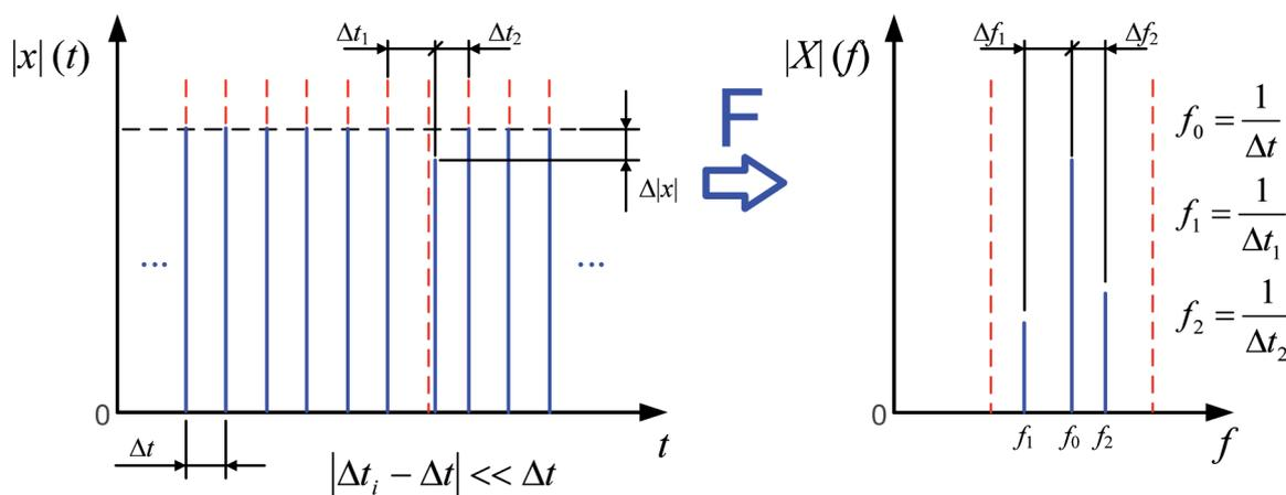
Fig. 9. The effect of one tooth defect in the time and frequency domains
