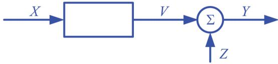
Fig. 3. System with the output disturbed by the process  $z$
