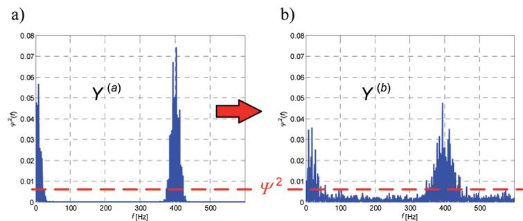
Fig. 2. The change of the spectral density of vibration accelerations of a defective rolling bearing without increasing the vibration level
