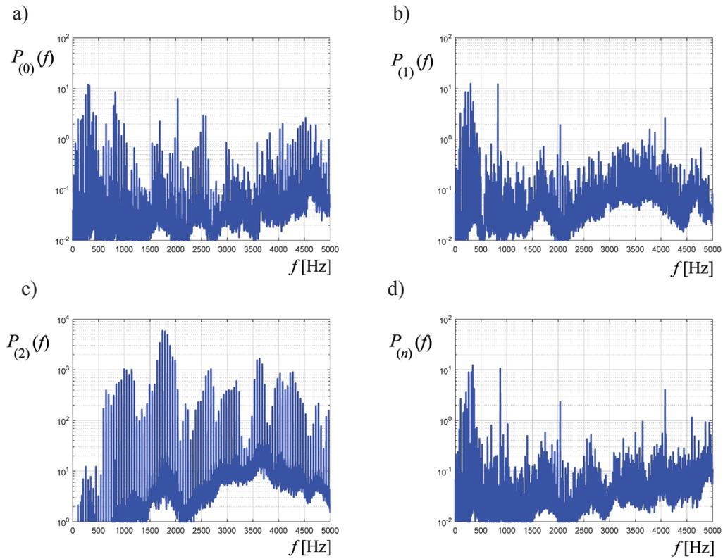
Fig. 4. Power spectrum density for the selected tests: a) maintenance state without defects, b) maintenance state with a slightly defected tooth, c) maintenance state with a strongly defected, d) maintenance state with a new wheel (not run-in)
