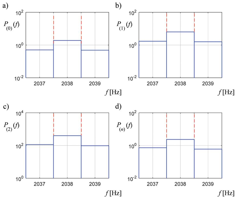
Fig. 5. The filtered bands of power spectrum in the vicinity of the mesh frequency: a) maintenance state without defects, b) maintenance state with a slightly defected tooth, c) maintenance state with a strongly defected, d) maintenance state with a new wheel (not run-in)
