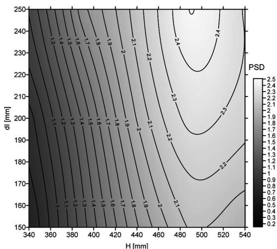
**Fig. 4.** The magnitude of the power spectral density *PSD* as a function of distance between electrodes *H* and distance between emission elements *dl* for a DELTA type electrode
