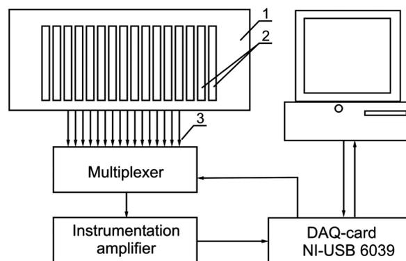
Fig. 2. Schematic of the circuit current density distribution measurements on the surface of the collecting electrode, 1 – collecting electrode, 2 – measurement fields, 3 – measurement signals
