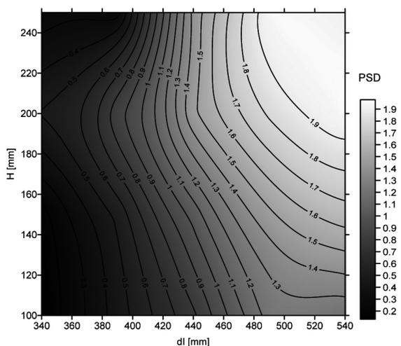
**Fig. 5.** The magnitude of the power spectral density *PSD* as a function of distance between electrodes *H* and distance between emission elements *dl* for a U-type electrode
