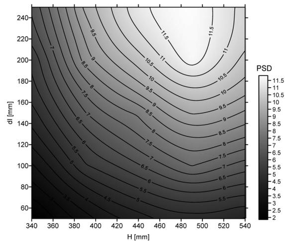
**Fig. 3. The magnitude of the power spectral density  $PSD$  as a function of the distance between electrodes  $H$  and the distance between emission elements  $dI$  for spike type electrodes**
