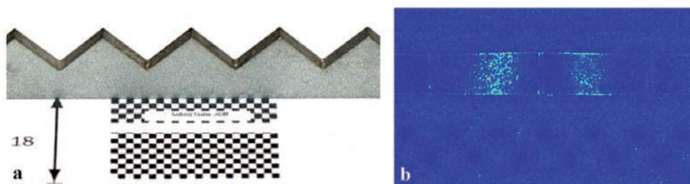
Fig. 6. The height standard used to construct a 3D image and an example of an image after segmentation that shows an area with good sharpness
