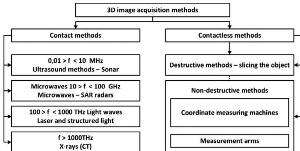
Fig. 1. Contact and contactless methods of 3D image acquisition
