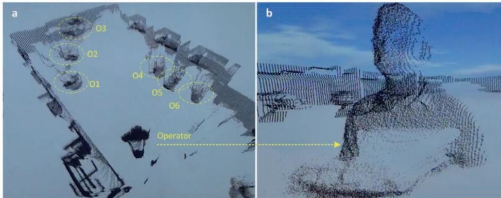
Fig. 4. A 3D image obtained using the TOF method (a) the entire room's image, (b) the operator's image
