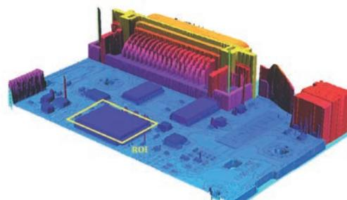
Fig. 12. An example of an electronic board's 3D image obtained by laser triangulation
