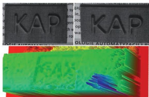
Fig. 8. A 3D image of the height standard built from a series of 25 2D images
