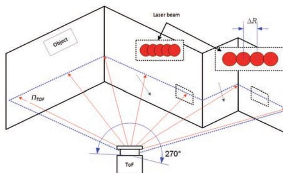
Fig. 3. Acquisition of a distance profile in the measurement plane  $\Pi_{TOF}$  on surfaces positioned at various distances from the measurement system
