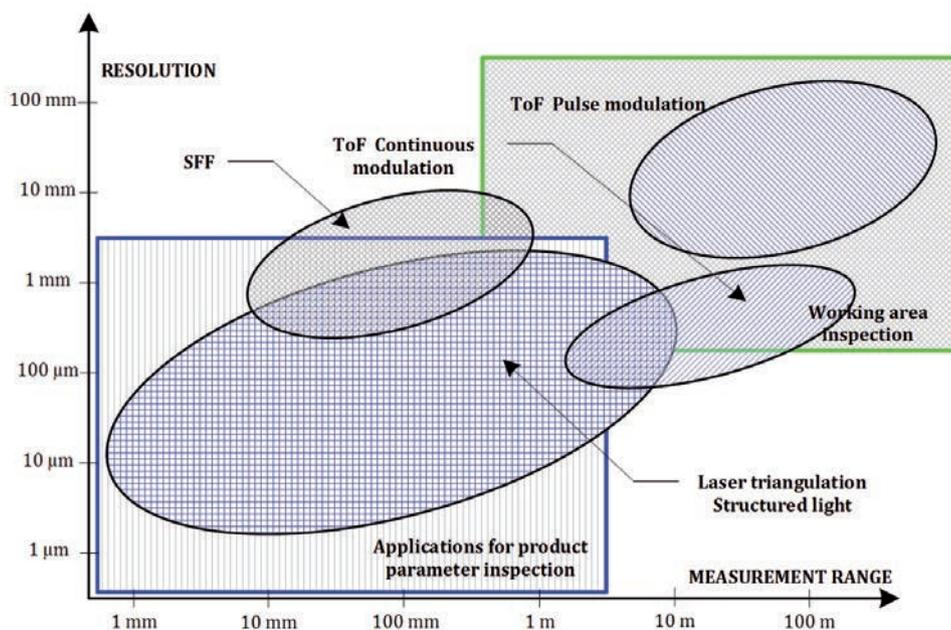
Fig. 14. The range of implementation of 3D systems to industry taking into consideration the measurement range and resolution of methods for construction of 3D images
