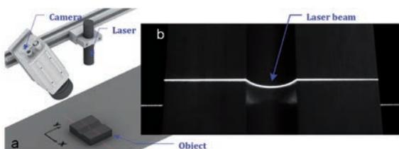
Fig. 10. Triangulation: a – Vision system configuration, b – Laser beam image registered by the camera
