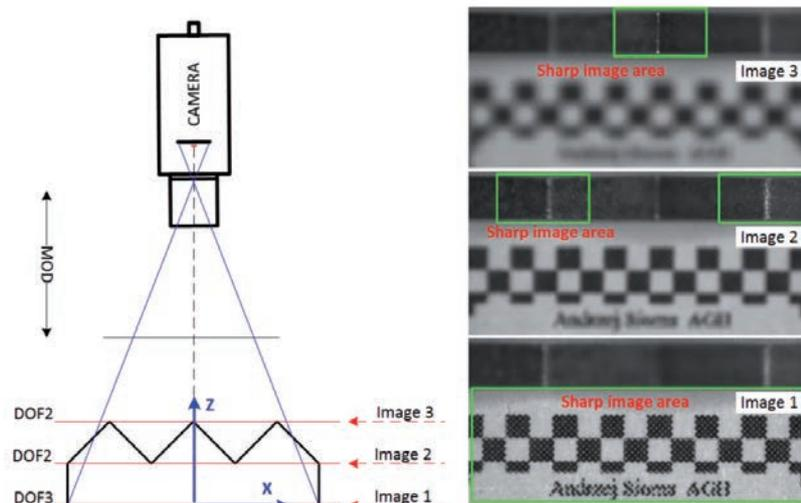
Fig. 5. A method for a 3D image acquisition based on DOF information
