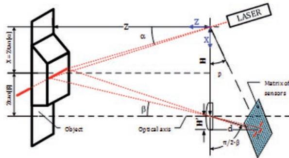
Fig. 11. Diagram of measurements taken with a laser beam and a 2D sensor matrix
