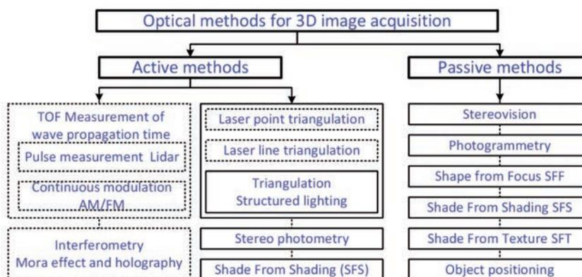
Fig. 2. Active and passive methods used for 3D image acquisition
