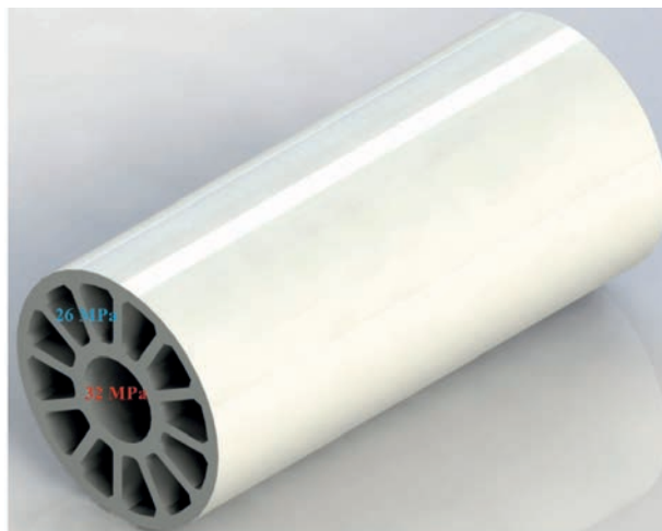
Fig. 1. Pressure in multichannel pipe during strength test
