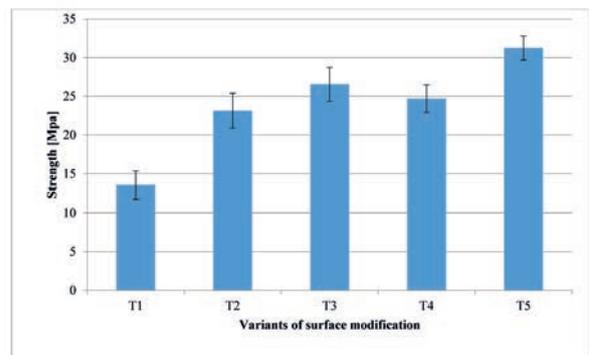
Fig. 5. Shear stress of 316L steel adhesive joint specimen bonded with Loctite EA 9466
