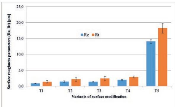
Fig. 4. The effect of surface treatment on the value of surface roughness parameters Rz and Rt
