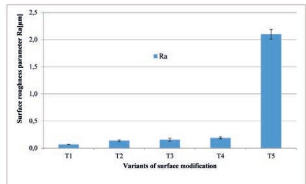
Fig. 3. The effect of surface treatment on the value of surface roughness parameter Ra
