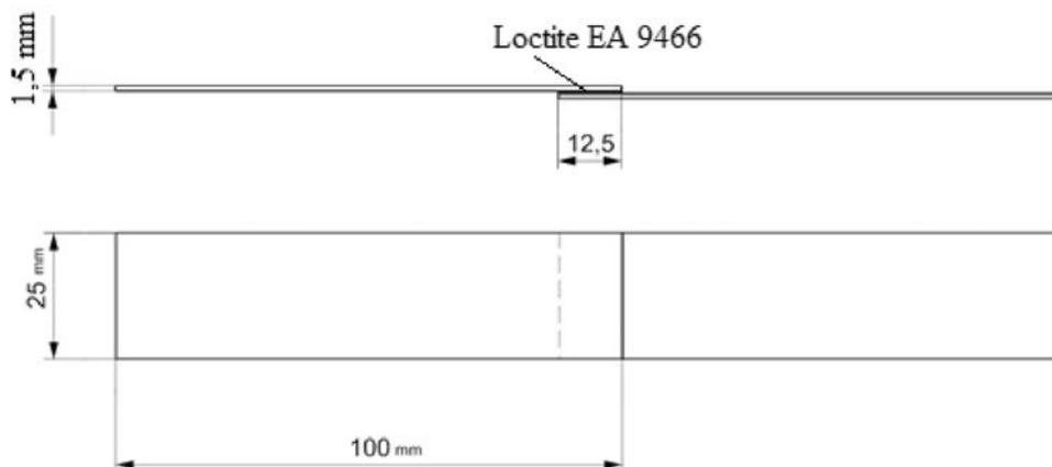
**Fig. 1. Schematic representation of the single lap adhesive joint**
