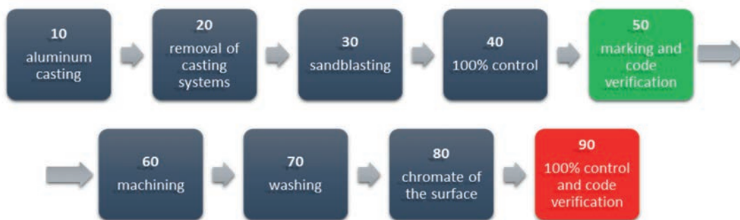
Fig. 5. Technological process of an aluminium part marked with Nd-Yag laser
