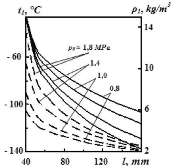
Fig. 7. Change of static temperature  $t_i$  (—) and density  $\rho_i$  (---) at length  $l$  of the broadening part of the nozzle at different pressure  $p_0$
