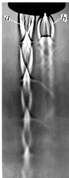
**Fig. 1.** Structure of supersonic air jets introduced to the atmosphere for *a*)  $n = 1.3$ , and *b*)  $n = 6.9$ . Critical diameter of the nozzle  $d_{cr} = 6 \text{ mm}$ , gas consumption by each nozzle  $V_n = 3.6 \text{ m}^3/\text{min}$
