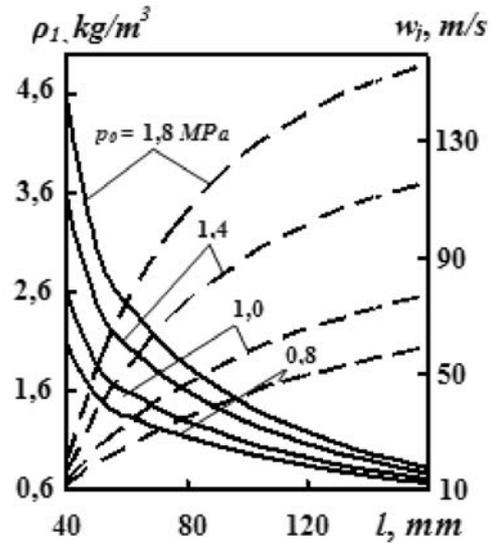
Fig. 6. Distribution of density  $\rho_i$  (—) and velocity of  $i$ -th particle  $w_i$  (---) at length  $l$  of broadening part of the nozzle at various entry pressure  $p_0$
