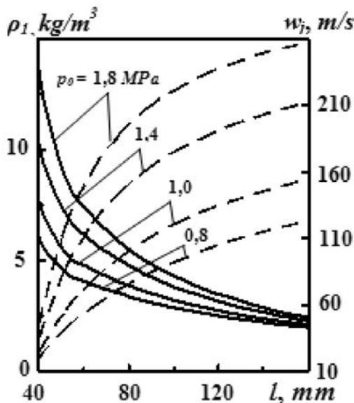
Fig. 5. Distribution of density  $\rho_i$  (—) and velocity of  $i$ -th particle  $w_i$  (---) at length  $l$  of broadening part of the nozzle at various entry pressure  $p_0$
