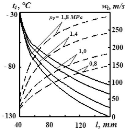
Fig. 4. Effect of pressure  $p_0$  on a change of temperature  $t_i$  (—) and velocity of  $i$ -th particle  $w_i$  (---) at length  $l$  of broadening part of the nozzle. Source data:  $\mu = 0.3$
