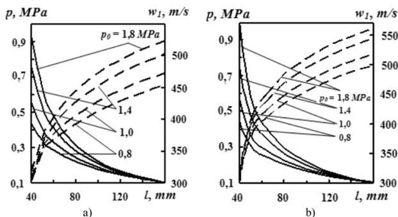
Fig. 3. Effect of pressure  $p_o$  on static pressure distribution  $p$  (—) and gas velocity  $w_1$  (---) in a function of length  $l$  of the broadening part of the nozzle. Source data: a)  $\mu = 1.5$ ; b)  $\mu = 0.3$
