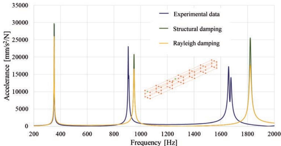
**Fig. 8. Frequency response function comparison for M05 beam**
