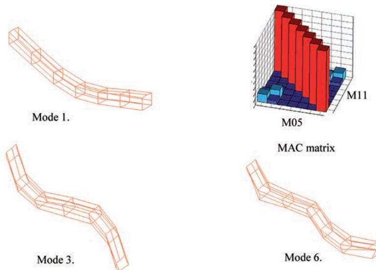
Fig. 4. Mode shapes visualization of 2 types of examined beams
