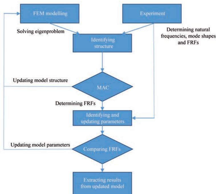
Fig. 2. Model identification procedure
