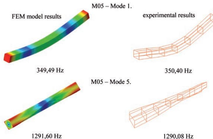
Fig. 7. Mode shapes comparison for M05 beam
