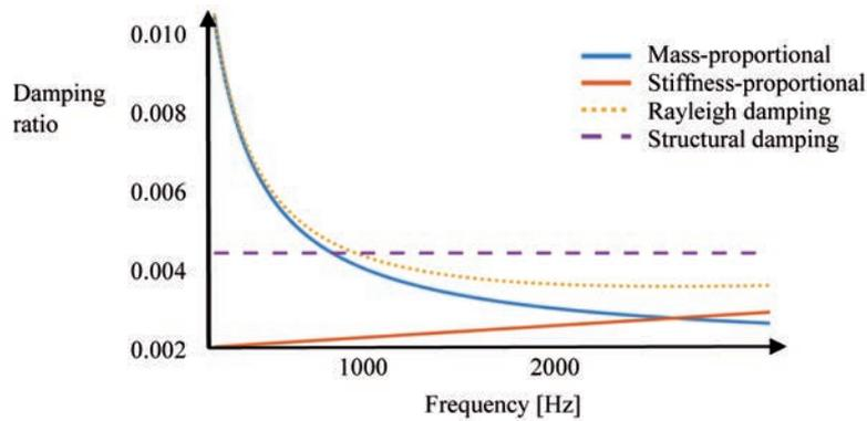
Fig. 6. Damping ratios derived from Rayleigh damping and structural damping model for M05 beam
