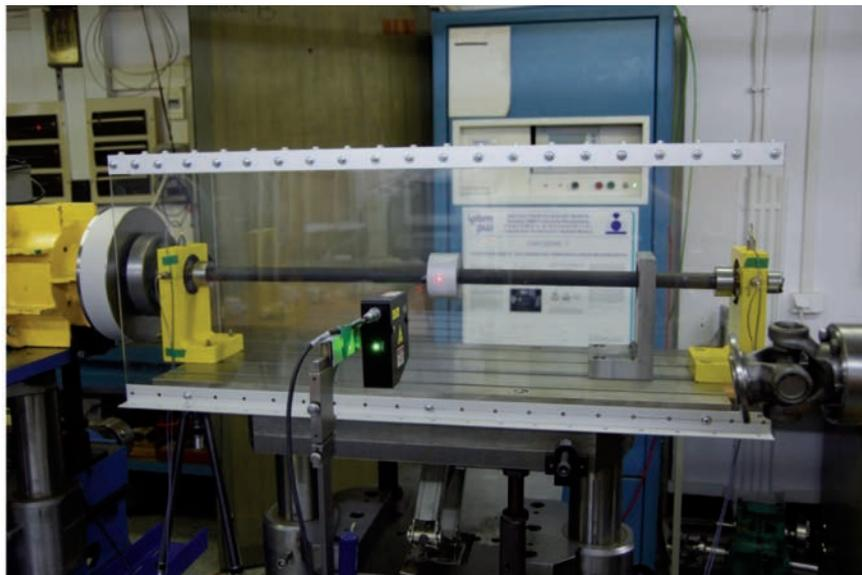
Fig. 1. Research set-up for testing critical velocities of shafts
